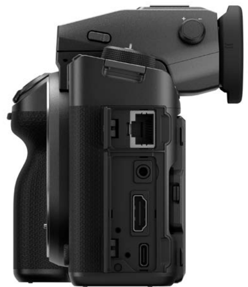
Full size HDMI Type A and USB-C connectors.
