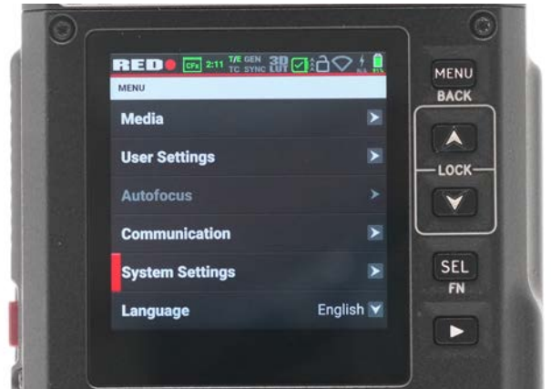
2. Push Menu button to go to home page. Navigate with Up and Down arrow keys and SEL to Select. Let's select System Settings.
