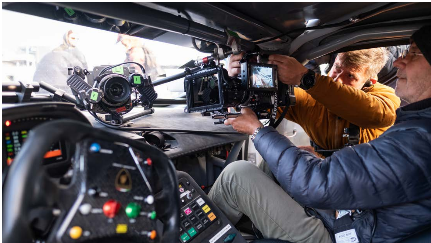
At center, RIALTO with Leica Summilux-M 0.8 35mm f/1.4 and Tilta Nucleus-M wireless lens control. At right, V-RAPTOR with Panaspeed.
