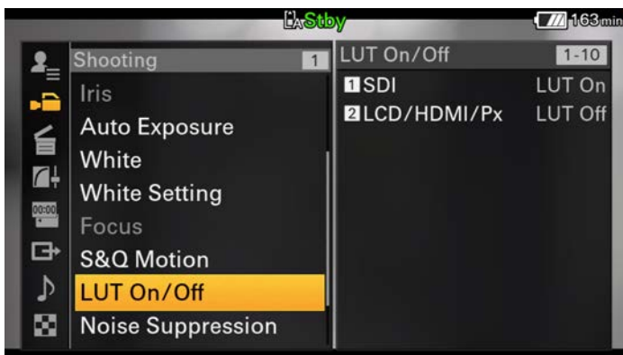
Turn LUT displayed on Monitor or EVF to On or Off.
