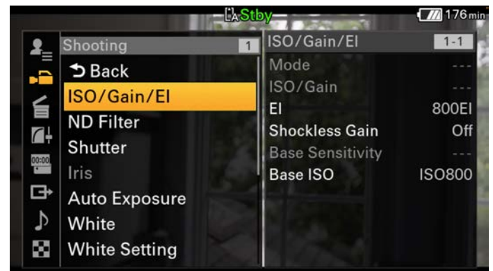
Base ISO of 800 or 3200. Shockless means smooth transition.
