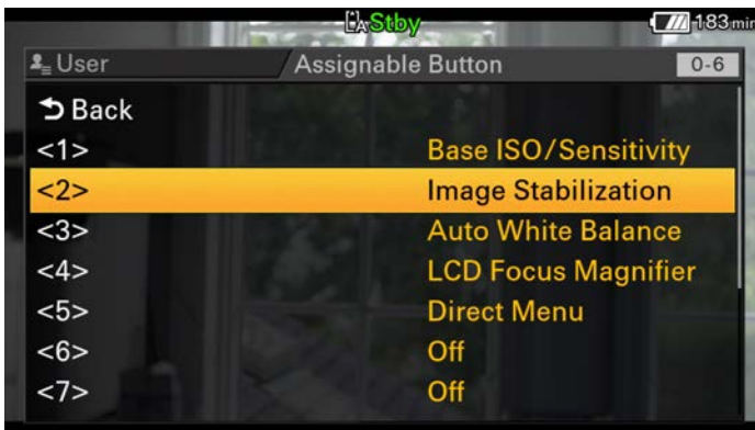
Assignable buttons are helpful. Use chart tape to identify on body.
