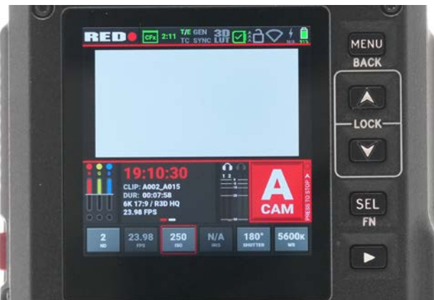
5. Seeing actual stops of light lost is nice—less math on set. Adjust ND, fps, ISO, iris, shutter and white balance directly on touch screen.
